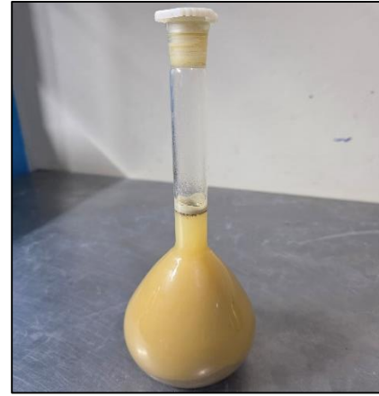
Fig. 5 Volumetric weight test
