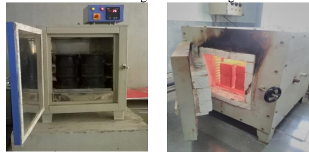
Fig. 4 Different states of the test apparatus for elevated temperature curing
