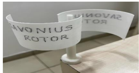
Fig. 10 A small-scale 3D printed model of the Savonius rotor by Poly-Lactic Acid (PLA)
