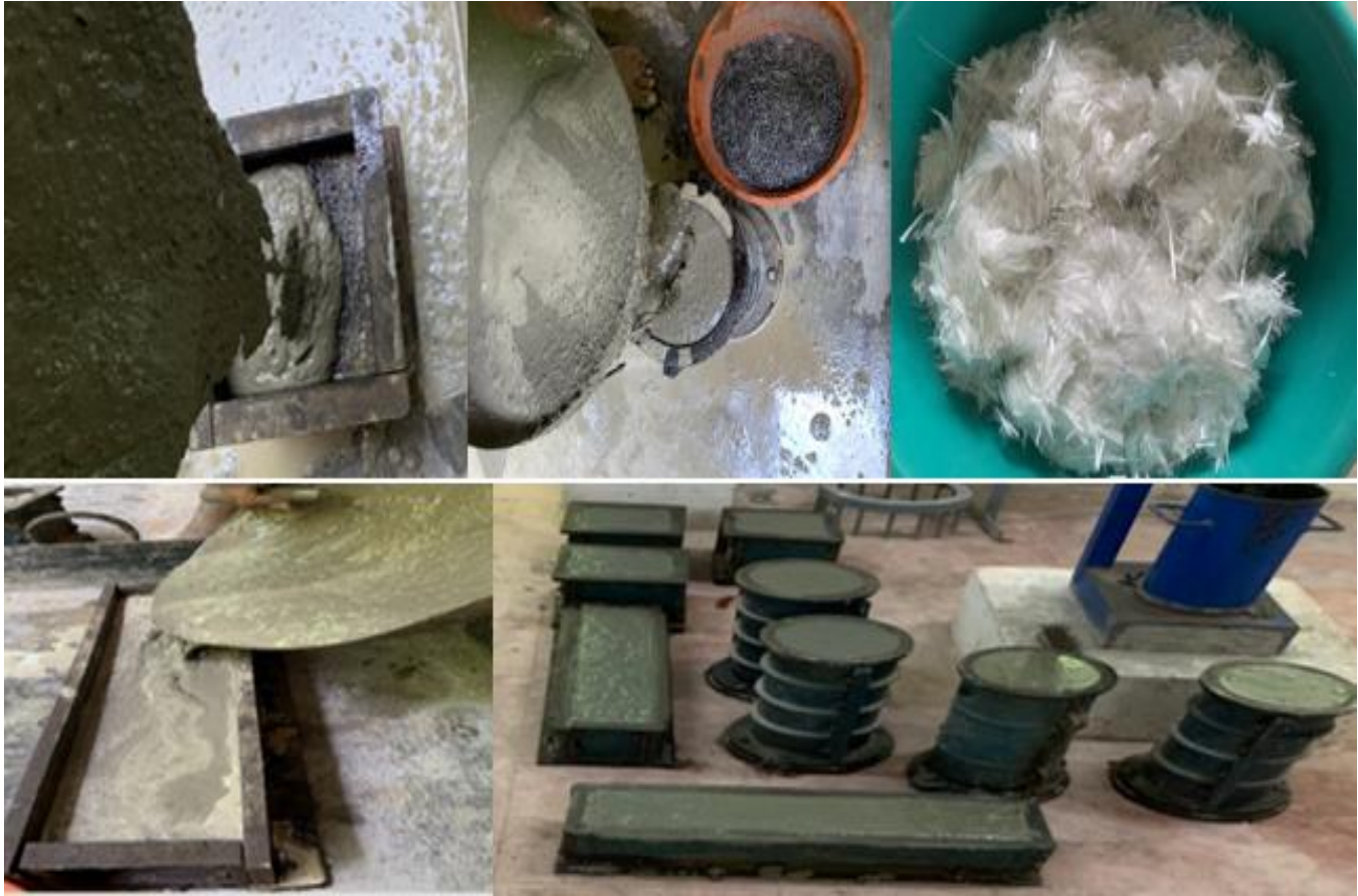
Fig. 4 Casting hybrid SIFCON specimens
