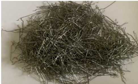
Fig. 1 Hooked-end steel fibres
