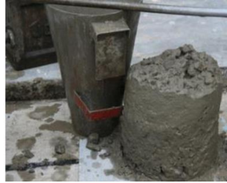
Fig. 6 Slump flow test for concrete
