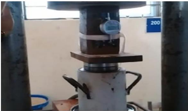
Fig. 9 Modulus of elasticity test of concrete
