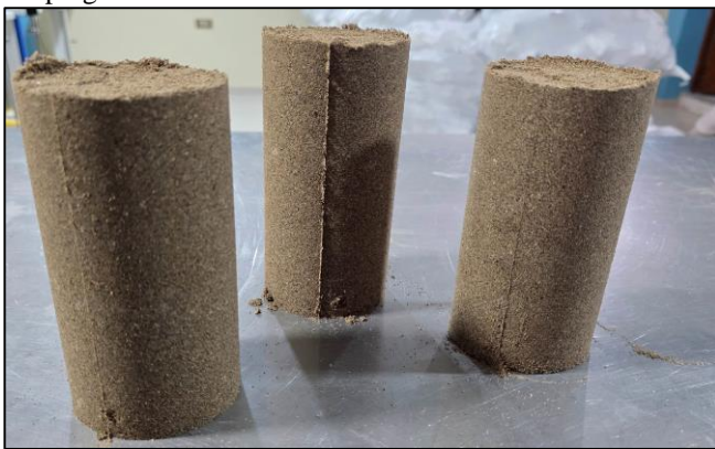
Fig. 17 Final specimens made by wet tamping
