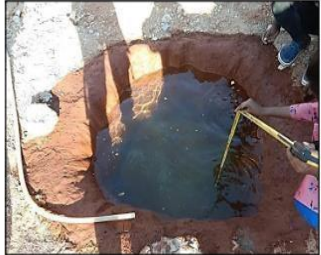
Fig. 17 Measurement of Seepage losses in pit
