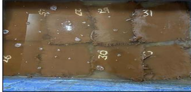
Fig. 13 Water Absorption testing on lab samples
