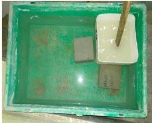
Fig. 6 Alkali activator solution placed in water bath
