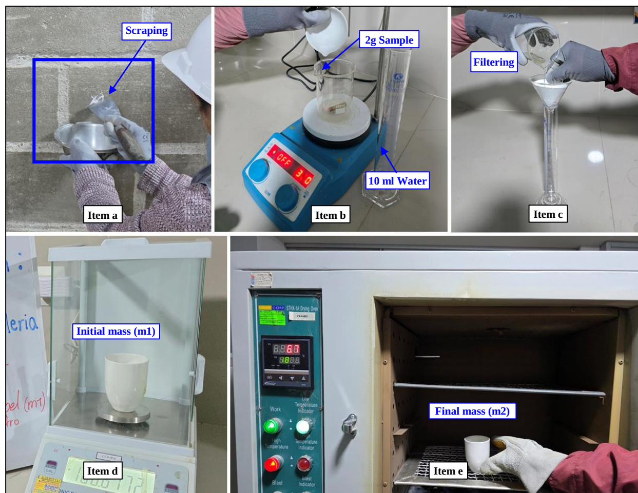
Fig. 16 Procedure for measuring soluble salts
