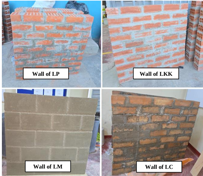
Fig. 13 Drying brick walls
