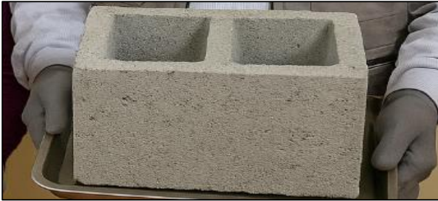
Fig. 6 Pacasmayo B14 concrete block
