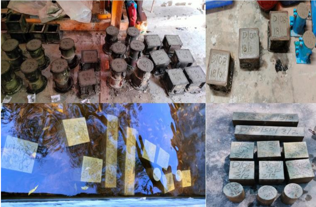
Fig. 6 Preparation, casting, curing, specimen arrangement for mechanical and durability testing of concrete mixes
