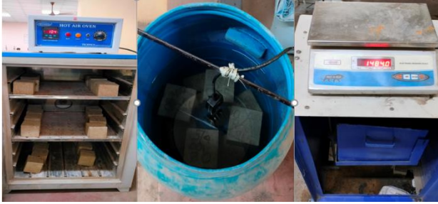
Fig. 12 Laboratory test procedure on absorption of water and density of concrete specimen
