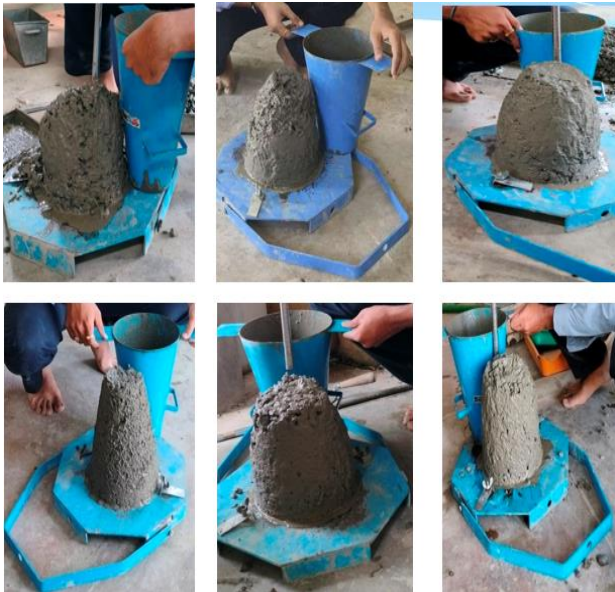
Fig. 4 Slump test appearance of concrete mixes at different replacement levels of Processed Overburden Sand (POBS)
