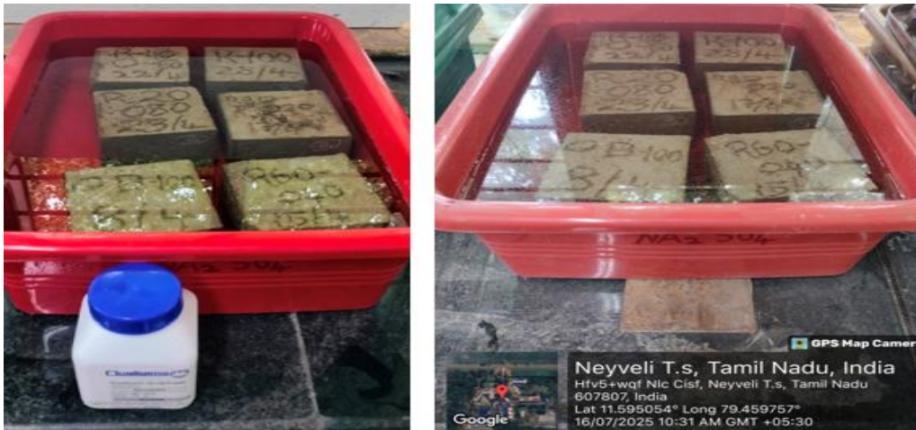
Fig. 22 Setup used for measuring sulphate resistance of concrete specimen in sodium sulphate ( \text{Na}_2\text{SO}_4 ) Solution
