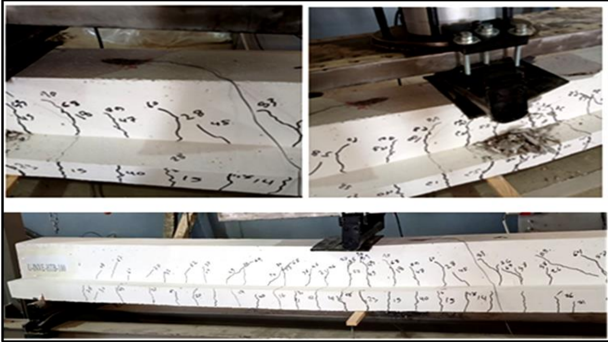
Fig. 14 Beam failure method (U- INVE-HTB - 100)
