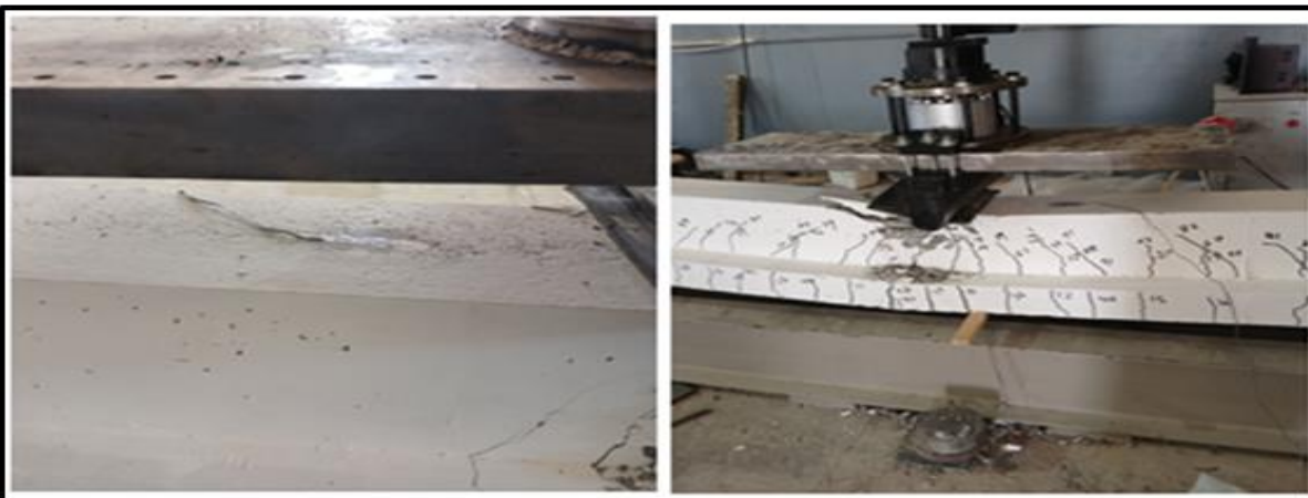
Fig. 13 Beam failure mode (U- INVE-HTB - 50)
