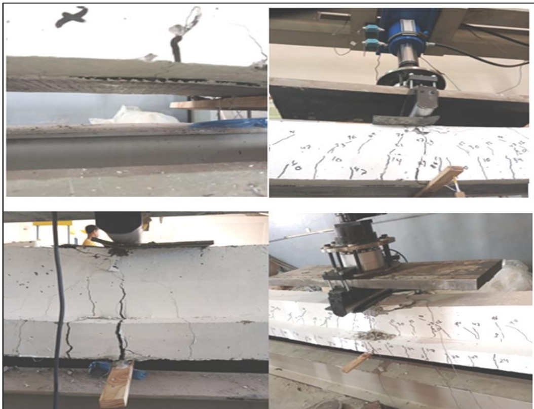
Fig. 16 Beam failure mode (ST- INVE-HTB-50)
