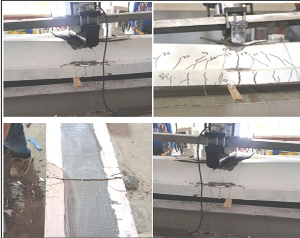
Fig. 15 Failure method of beam (ST- INVE-HTB-0)
