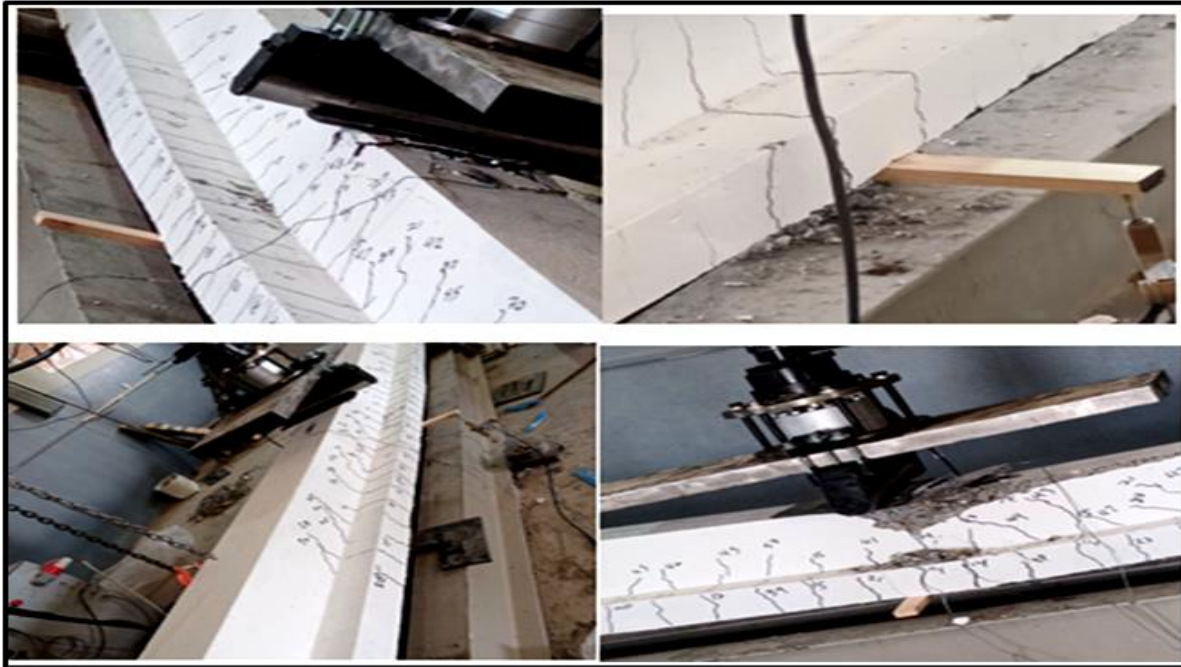
Fig. 12 Beam failure mode (U- INVE-HTB-0)
