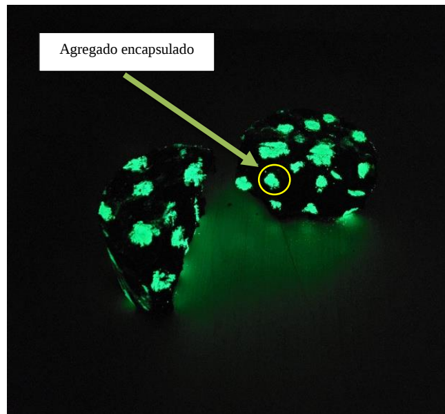
Fig. 14 Aggregates encapsulated by Asphalt cement
