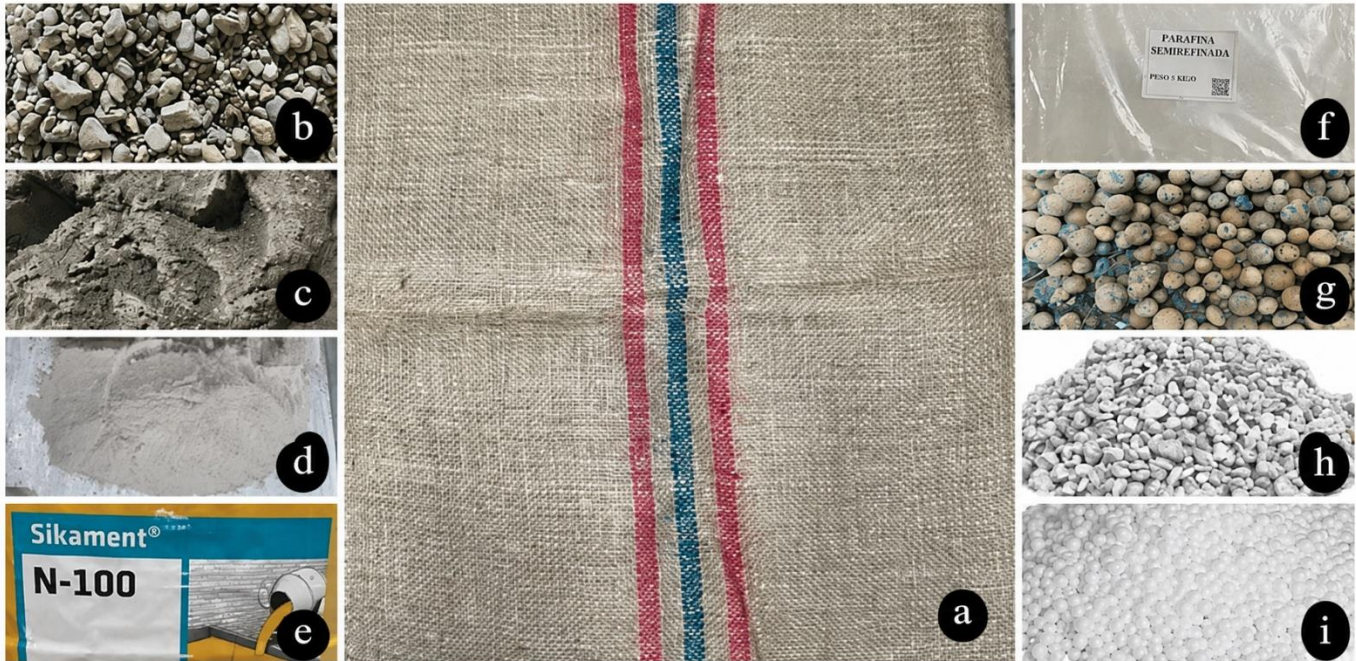
Fig. 2 Materials: (a) Sisal fibers, (b) AG, (c) AF, (d) Filler, (e) Superplasticizer, (f) Paraffin, (g) Arlite, (h) Pumice, (i) Polystyrene.
