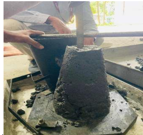
Fig. 3 Slump test of fresh concrete
