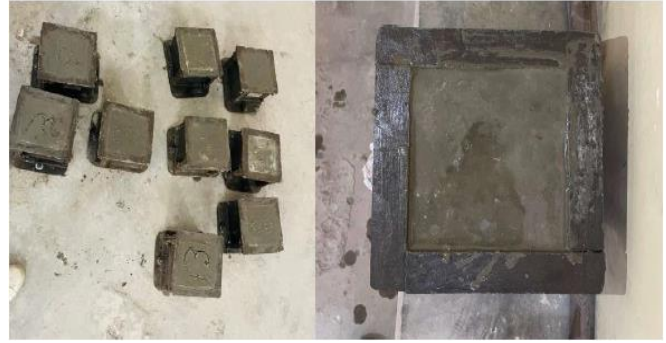
Fig. 2 Preparation and casting of concrete cube specimens for compressive strength testing
