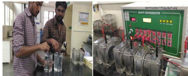
Fig. 18 Experimental setup for RCPT and preparation of electrolyte solutions for bacterial concrete specimens
