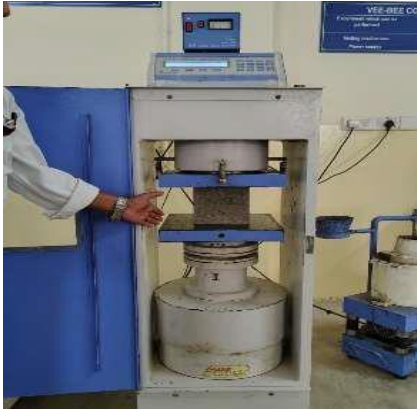
Fig. 4 CTM used for determining the compressive strength of specimens
