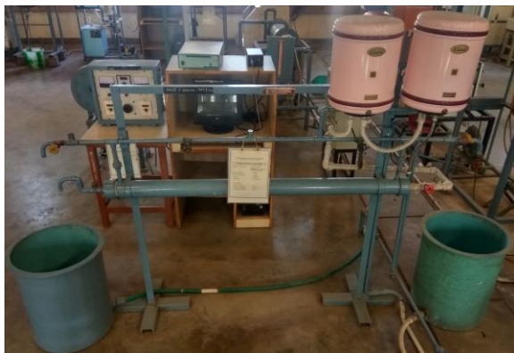
Fig. 1: Counter Current Double Pipe Heat Exchanger
