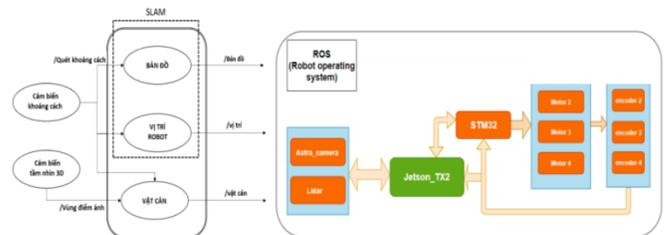
Figure 2: ROS-based perception system and hardware configuration of the robot system
