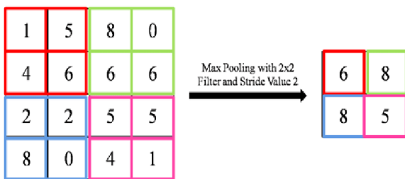
Figure 4: Max Pooling by 2X2
