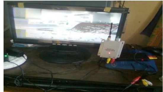
Fig 3: Receiving section contains PC, RF receiver with antenna, XGA TV box.
