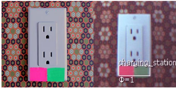
Fig.4 A Color Code (pink and green) Stuck on a Socket, to Mark a Charging Station
