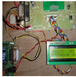
Fig.7. Testing soil moisture using Sensor
