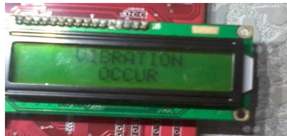
Fig 6: Vibration Sensor Detects the Vibration and Displays “Vibrations Occur”.
