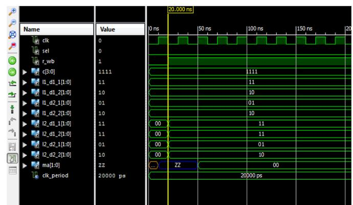
Fig 5. Simulation result of area efficient TCAM
