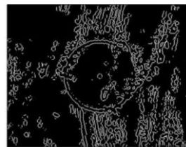
Fig. 7: Output of Laplacian of Gaussian Operator on connector endface profile.
