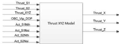
Fig.8. Input and Output Model for Thrust XYZ
