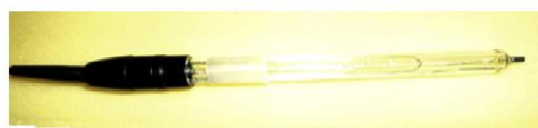
Fig .1: Physical Appearance of the ORP Sensor
