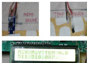
Fig 6 MEMS Sensor & Temp Sensor
