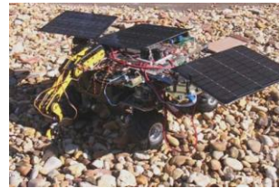
Fig.1.VANTER: a Solar-Powered Robotic Vehicle
