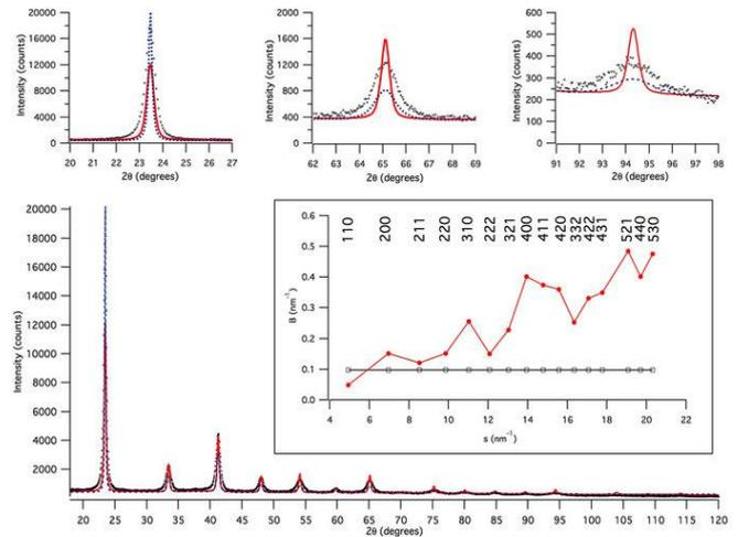
Fig. 2 To 5 XRD Peak Profile of Ground Sample for Downfeed (µm) -10, 30, 40 And 60
