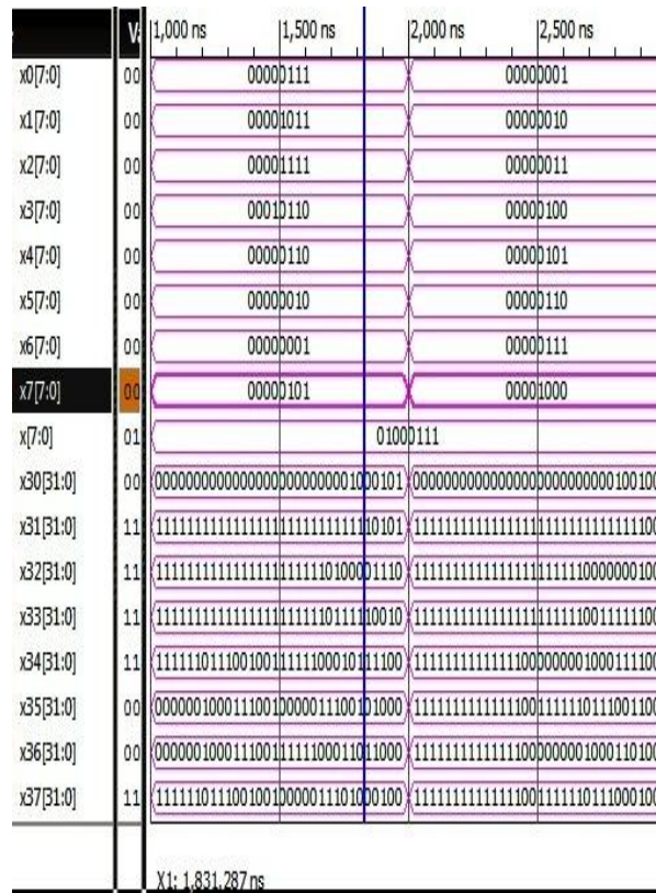
Fig 8: Simulation Results of Fast Fourier Transform using Baugh-Wooley Algorithm and Twin Precision technique.
