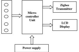
Fig. 3.1 Block Diagram of Transmitter
