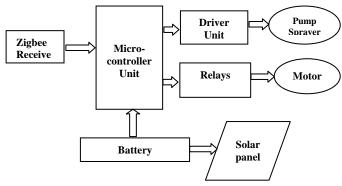
Fig.3.2 Block Diagram of Receiver
