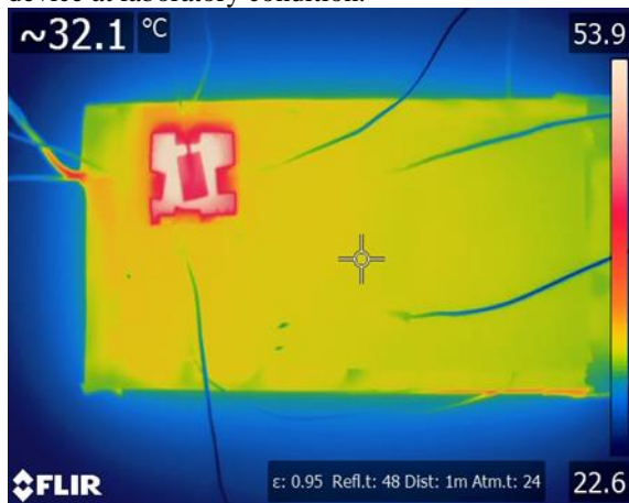
Figure 5: IR image of test device with IR material in the enclosure.
