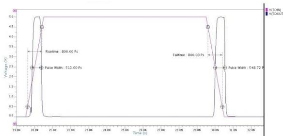
**Fig 13: Transition Detector Implementation-2, output response**
