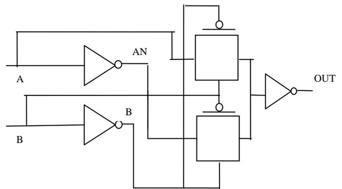
**Fig 16: Pass-Transistor XOR gate Schematic**
