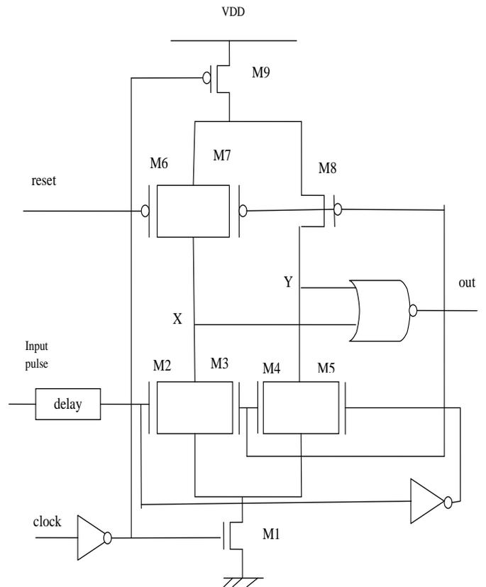
Fig 18: Stability Checker Implementation Schematic
