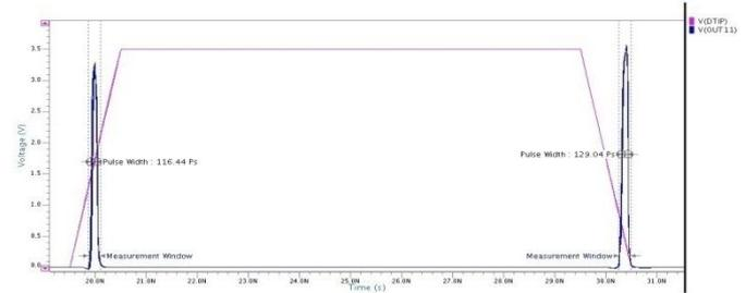
**Fig 10: Transition Detector - Implementation 1, output response for PVTA variations**
