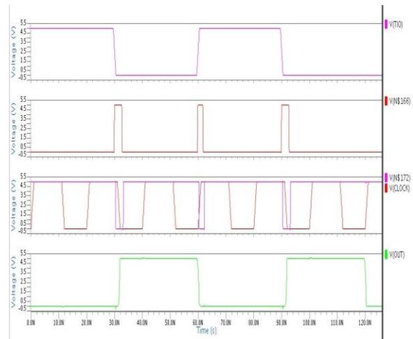
Fig 22: NOR Based Implementation output response
