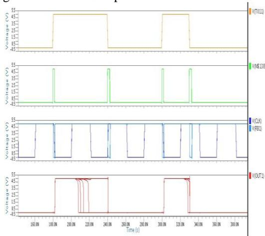
Fig 20: Stability Checker Implementation, output response with PVT variations
