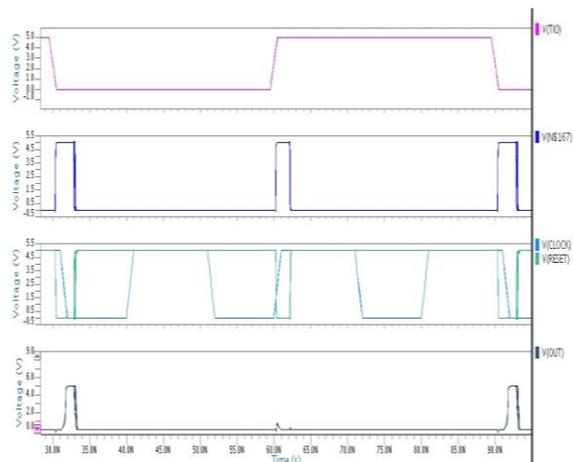
Fig 23: NOR Based Implementation output response with PVT variations
