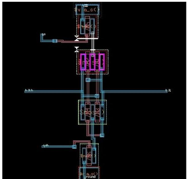
Fig 27: Sense Amplifier layout
