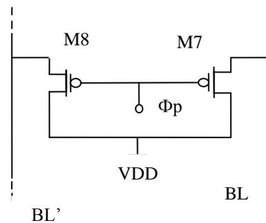
Fig 4: Pre-charge Schematic
