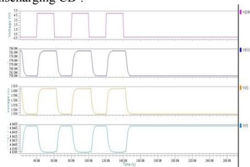
Fig 2: SRAM read operation
