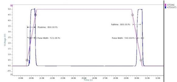
**Fig14: Transition Detector Implementation-2, output response for PVTA variations.**
