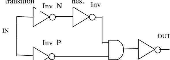
**Fig 8: Transition Detector - Implementation 1 schematic.**
