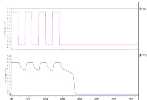
Fig 3: SRAM write operation
