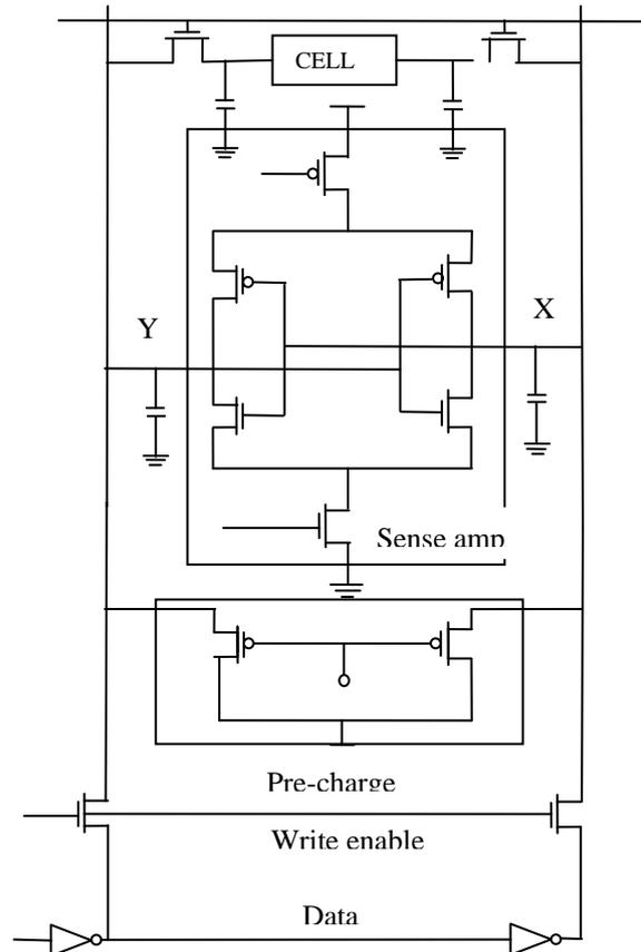
**Fig 6: Complete SRAM Schematic**
