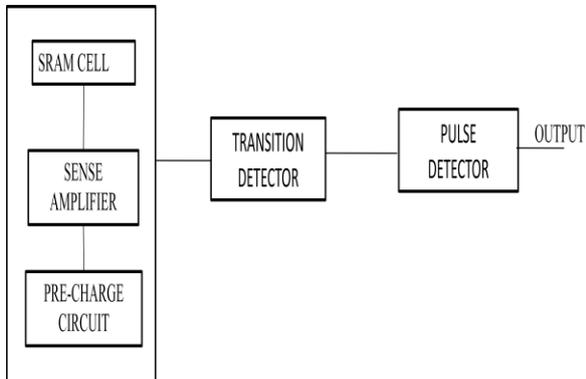
Fig 24: Complete Sensor block diagram
