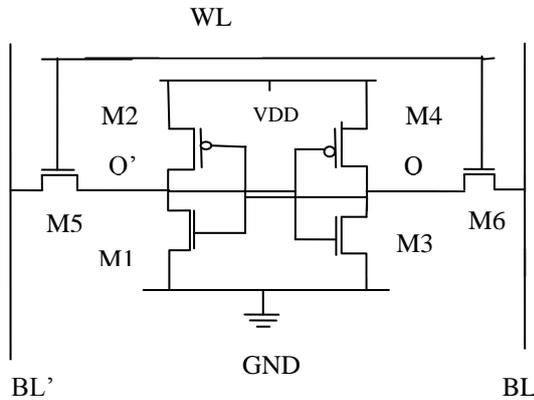
Fig 1: CMOS 6T SRAM cell
