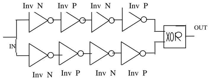
**Fig 15: Transition Detector – Implementation-3, schematic**
