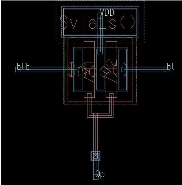
**Fig 28: Pre-charge circuit layout**
