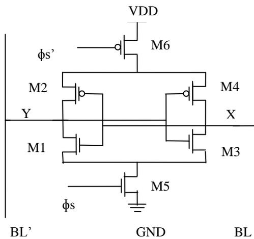
**Fig 5: Sense Amplifier Schematic.**
