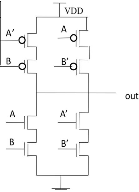
**Fig 11: CMOS XOR gate schematic**
