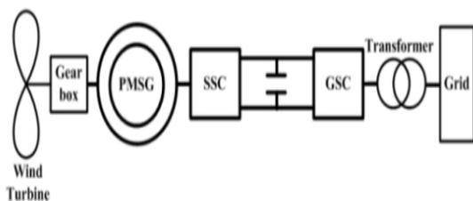
Fig-14. General structures of PMSG WECS connected to the grid
