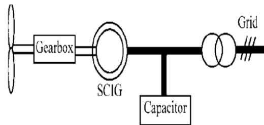
**Fig-2. Scheme of a fixed speed concept with SCIG system**
