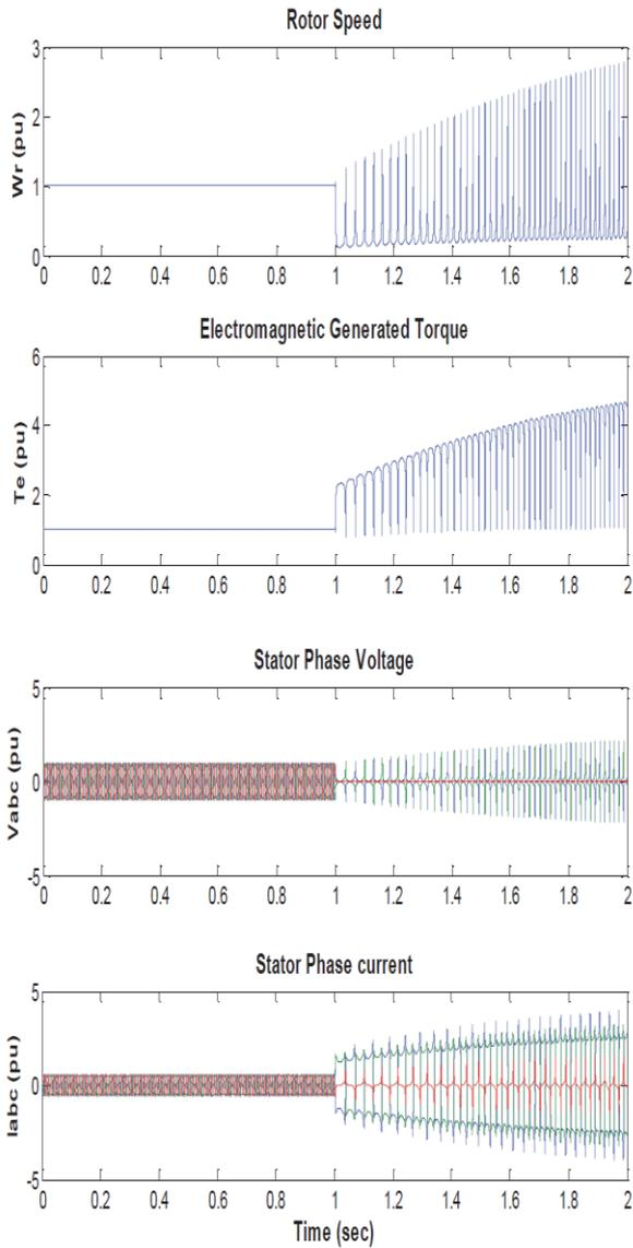
Fig-7. The response of PMSG to a short circuit fault
