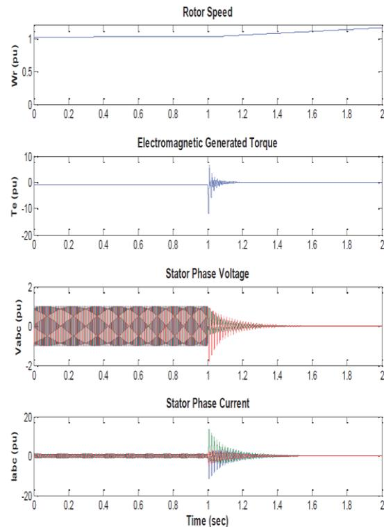
Fig-6. Response of self-excited SCIG to short circuit fault
