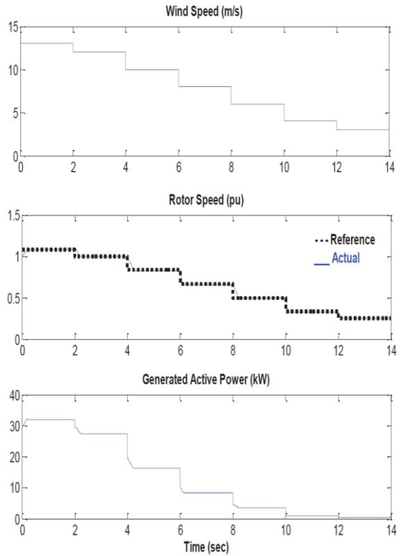
Fig-8. MPPT response and generated power in PMSG
