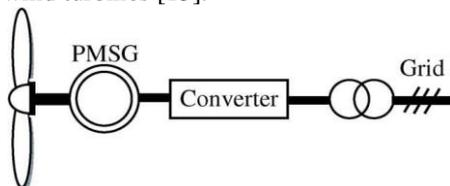
Fig-3. Scheme of a direct-drive PMSG system
