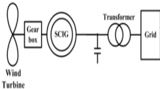
Fig-13. SCIG Grid-Connected
