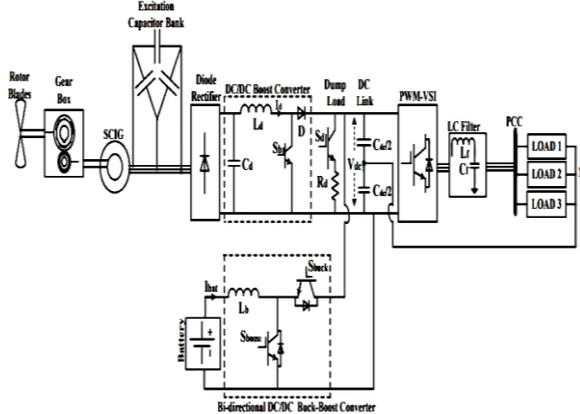
Fig-11. Stand-alone SCIG-based WECS
