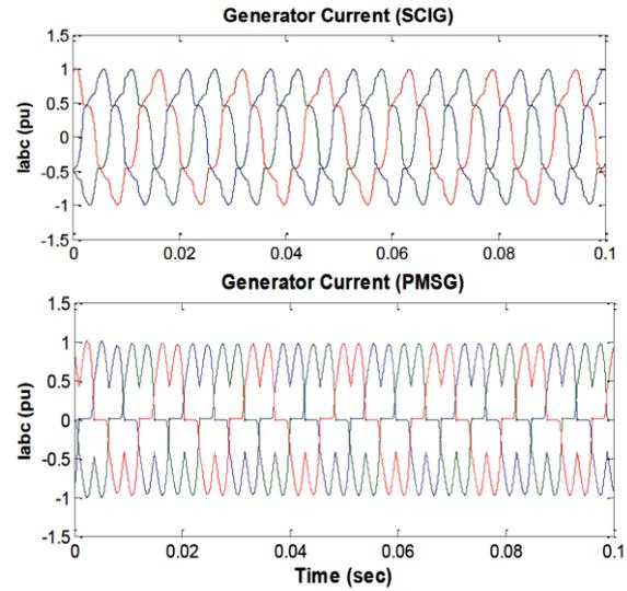
**Fig-10. Generator stator currents at rated wind speed**
