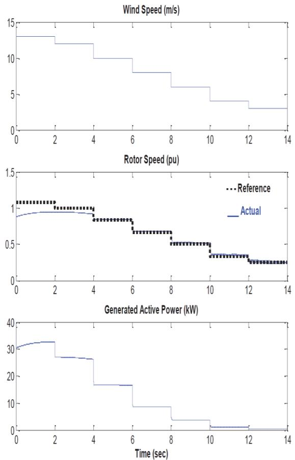
Fig-9. MPPT response and generated power in SCIG
