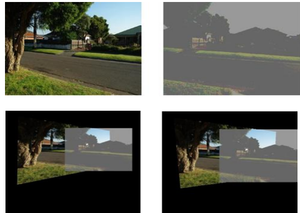
Fig. 2. Mosaicing results under illumination environment. Images to be stitched (a) noise-free image and (b) noisy image. Stitched image from methods based on (c) Euclidean distance, (d) Bound energy based matching.
