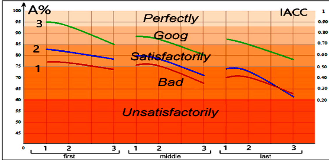
Fig. 3: Interaural correlation coefficients of the IACC (1) of the speech signal and the value of the articulation percentage A% (2), the IACC value of the pulse signal (3) on the listening positions in the room Different shades of color and lead letters indicate the legibility classes
