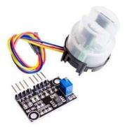
d) ELECTRICAL CONDUCTIVITY SENSOR: Salinity is the measure of the concentration of dissolved salts in water. Salinity is a ratio and not a physical parameter that can be measured. Thus. "Salinity sensors" do not exist, but the one which refers to as a salinity sensor is, in fact, a conductivity sensor.
