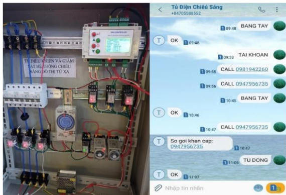
Fig. 12 (a)The controller cabinet and (b) SMS messages and communication calls between the device and the manager.
