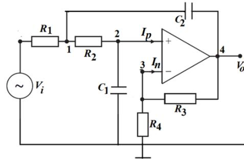
**Figure 2 Circuit for example 3,**
