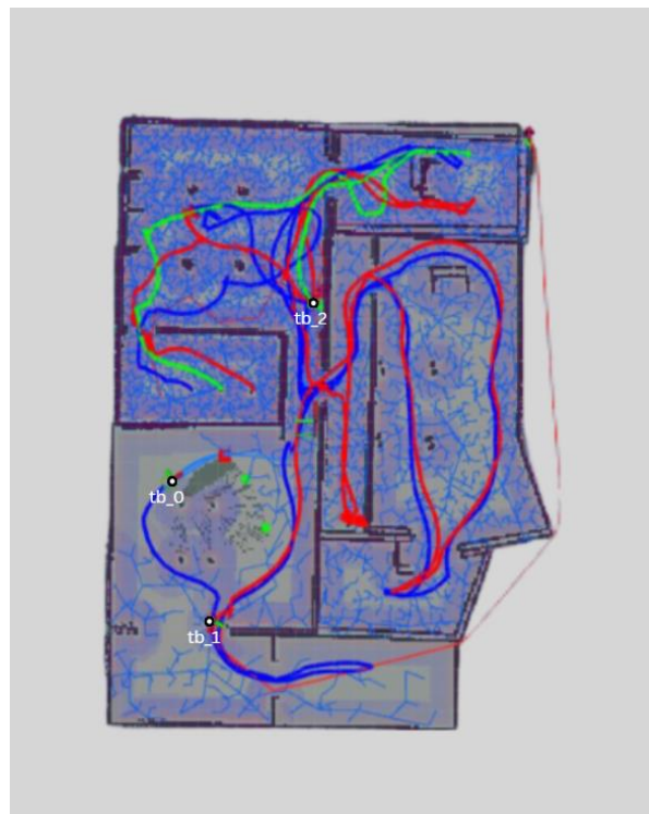
Fig. 7 Trial 3 output of the task allocation algorithm without the coverage penalty parameter (Umari et al. [28, 29]). Exploration travel path trajectories of robots: Robot 0 (blue), Robot 1 (red), and Robot 2 (green)
