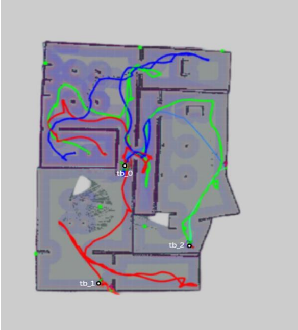
Fig. 9 Trial 2 output of proposed task allocation algorithm with coverage penalty parameter, Exploration travel path trajectories of robots: Robot 0 (blue), Robot 1 (red), and Robot 2 (green)
