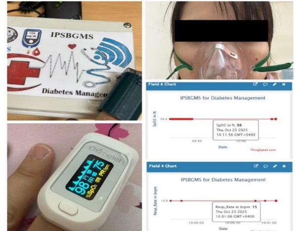
Fig. 8 SpO2 and RR readings from the IPSBGMS prototype and a commercially available tomorotec pulse oximeter
