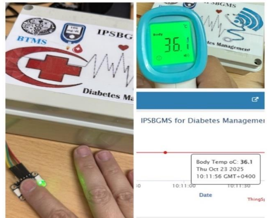
Fig. 9 BT readings from the IPSBGMS prototype and the medical-grade infrared thermometer
