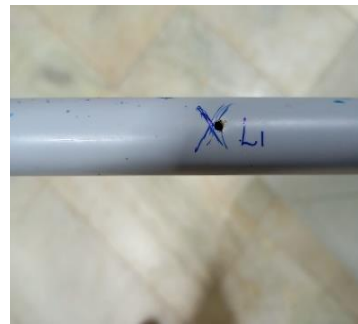
Fig. 16 Gas pipe indicating leakage point L 1
