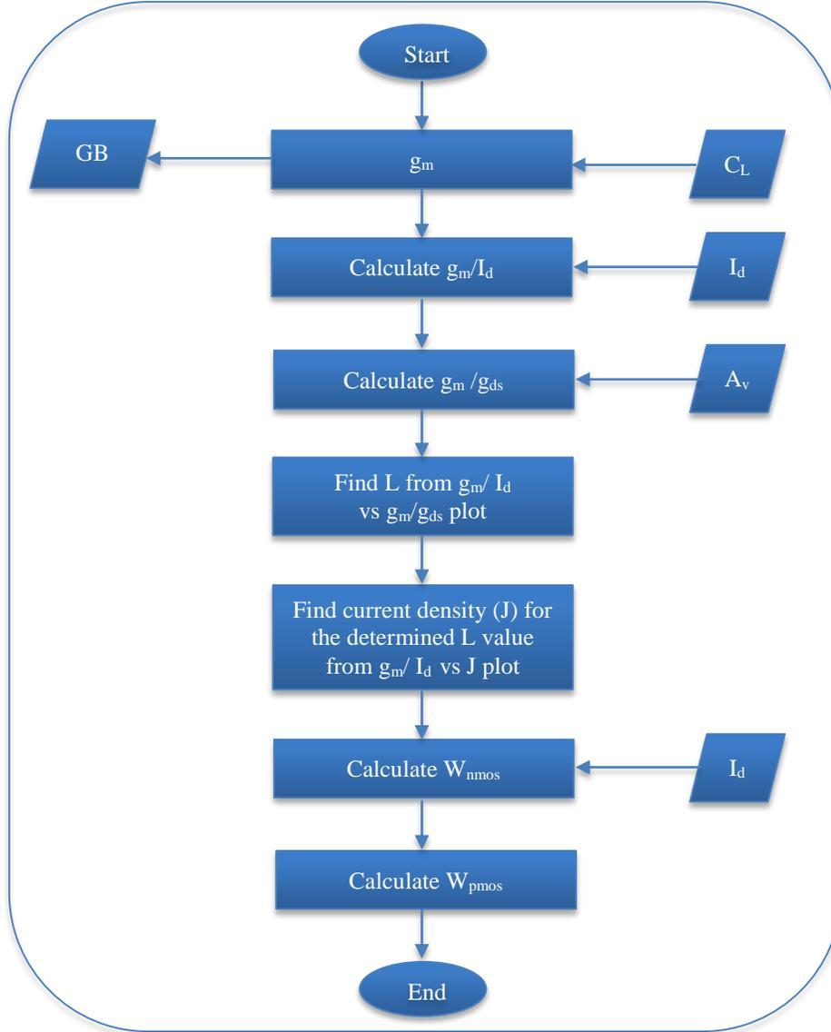
Fig. 5 The flow diagram illustrates the various stages of the k-NN methodology in designing the common source amplifier circuit
