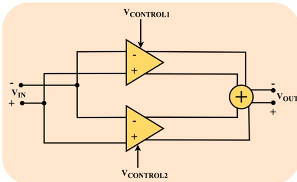
**Fig. 1** Block diagram representing the variable gain amplifier using the gilbert cell configuration blocks
