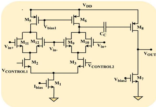
Fig. 6 Schematic of VGA using the gilbert cell configuration and common source amplifier
