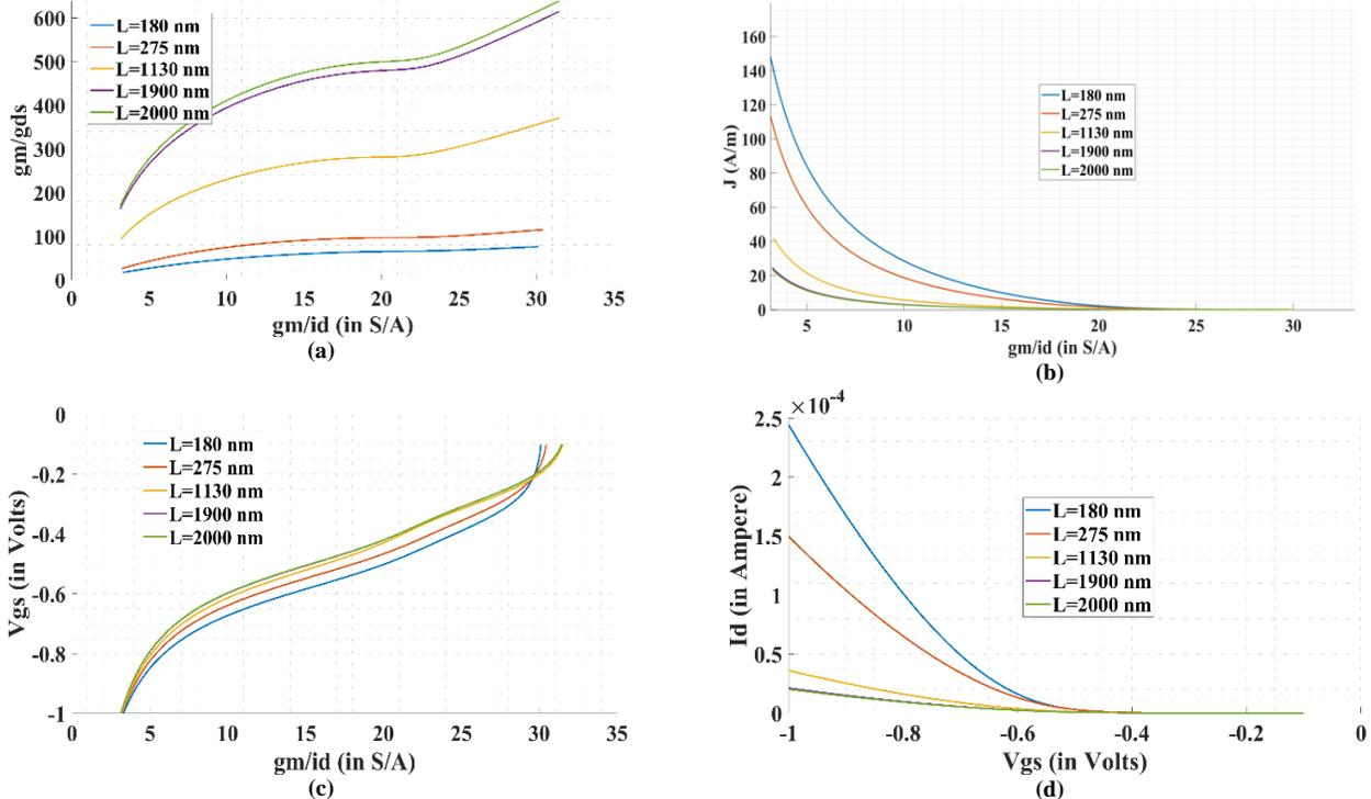
Fig. 3 Different plots plotted with respect to  $g_m/I_d$  for PMOS transistor (a)  $g_m/I_d$  Vs  $g_m/g_{ds}$ , (b)  $g_m/I_d$  Vs  $J$ , (c)  $g_m/I_d$  Vs  $V_{gs}$ , and (d)  $V_{gs}$  Vs  $I_d$ .
