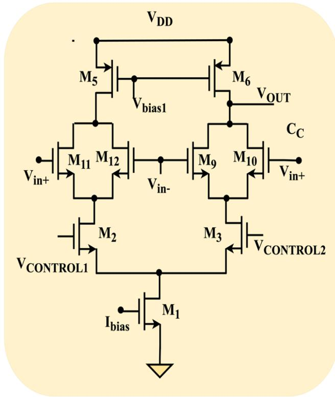
Fig. 4 Schematic of VGA using the gilbert cell configuration
