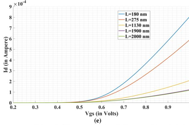
Fig. 2 Different plots plotted with respect to  $g_m/I_d$  for NMOS transistor (a)  $g_m/I_d$  Vs  $g_m/g_{ds}$ , (b)  $g_m/I_d$  Vs  $J$ , (c)  $g_m/I_d$  Vs  $V_{gs}$ , (d)  $g_m/I_d$  Vs  $V_{dsat}$ , and (e)  $V_{gs}$  Vs  $I_d$ .
