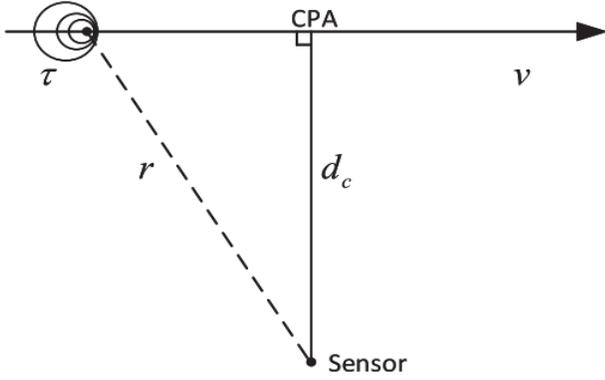
Fig. 3 A moving source radiating the signal with a constant frequency  $f_0$
