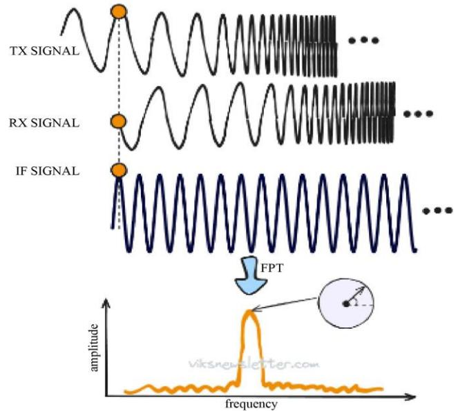
Fig. 2 Signal Estimation with CRT
