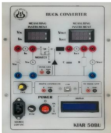
Fig. 5 The buck converter training kit
