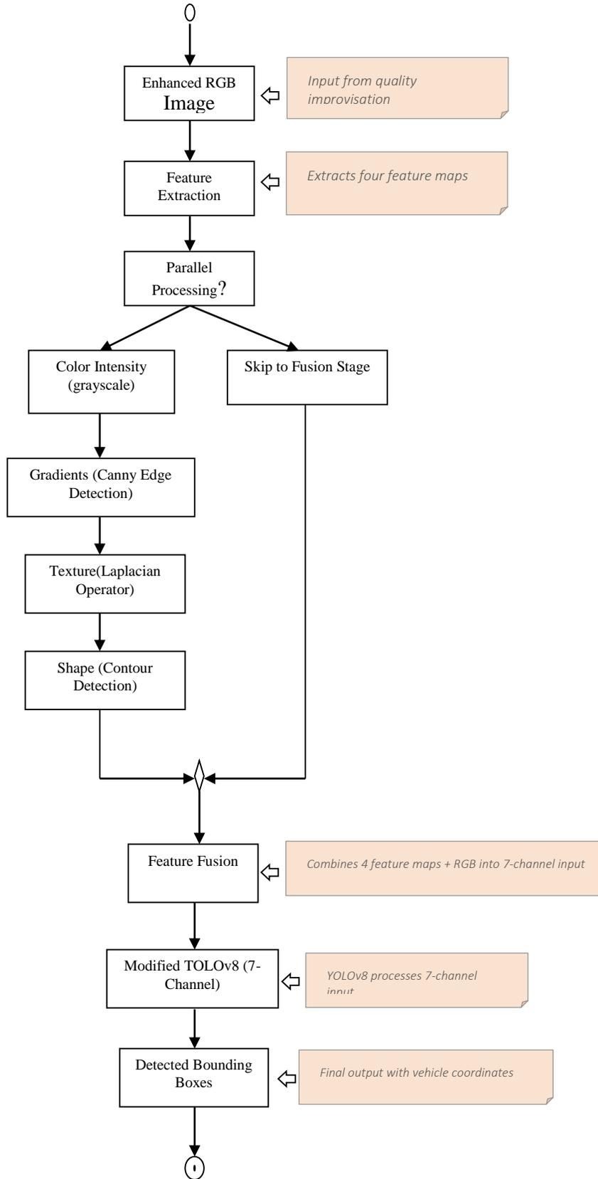
Fig. 8 Vehicle detection pipeline
