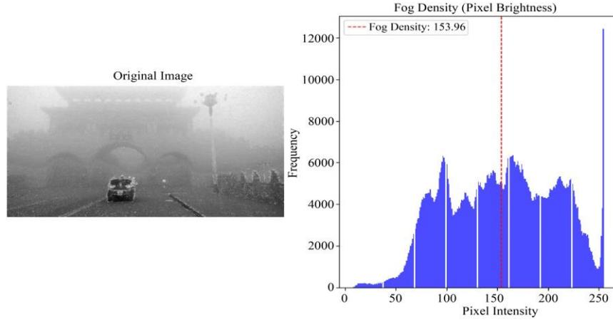
Fig. 11 Fog density with pixel brightness
