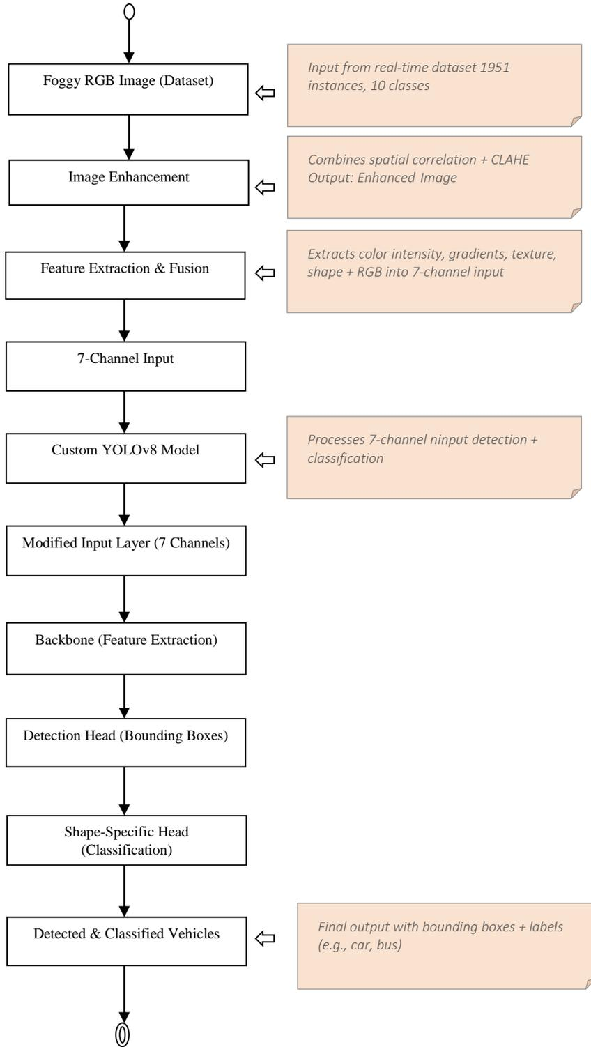
Fig. 9 Architecture diagrams of the proposed foggy vehicle
