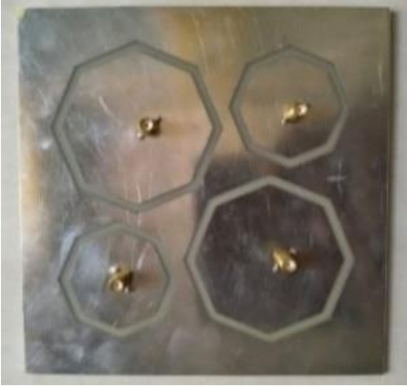
Fig. 6 Fabricated antenna back view showing SMA connectors integration and segmented ground
