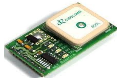
Figure 2: GPS Receiver MT 3318 Cirocomm
