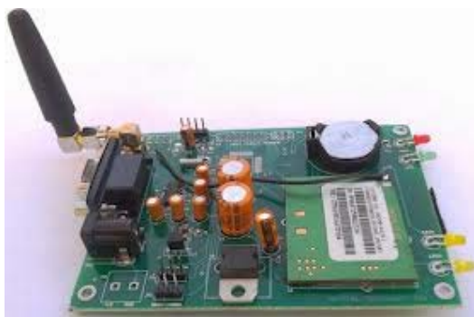
Figure 3:GSM Modem SIM 300
