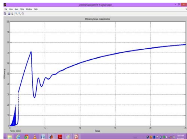
Fig 12. Efficiency vs Load Torque in armature voltage speed control of DC motor
