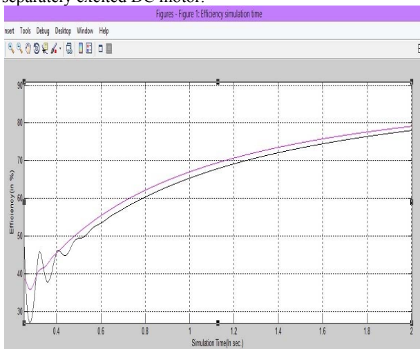
Fig 13. Comparison efficiency of armature control and armature field control of DC motor
