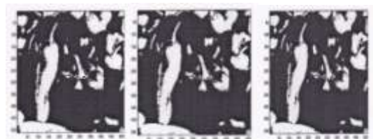
Rate – 1:5 Rate – 1:29 Rate – 1:67 Figure 20B) LSB based retrieved watermark after JPEG2000 compression
