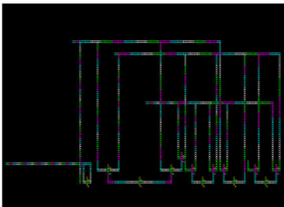
Fig. 7 Automatically Generated Layout for Binary To BCD Code Converter
