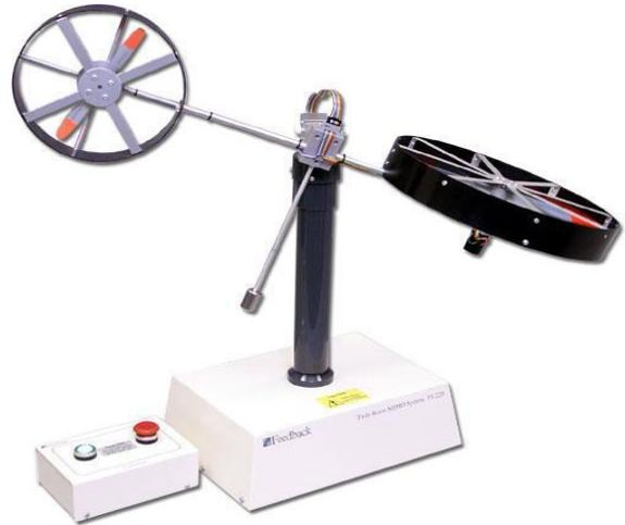
Figure 1. Twin Rotor MIMO System
